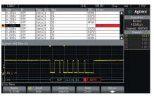
500 CAN serial packets over 9 seconds, captured at a high sample rate, using the 3000 X-Series's segmented memory
